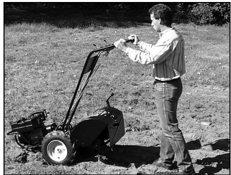
Figure 4-4: Find balance point before turning.
